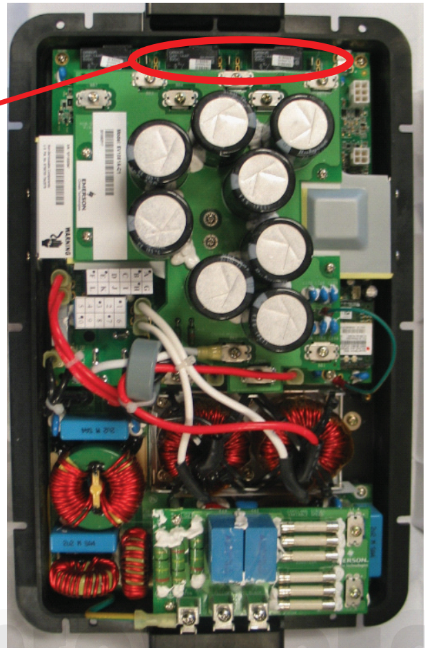
Fig. 23 – High Voltage Input-Output Connections on Drive
