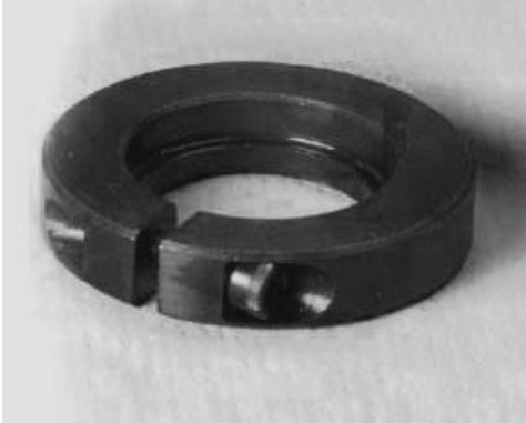
Fig. 7 – Tightening Locking Collar
