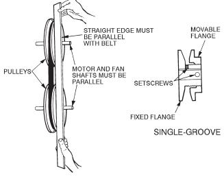
Fig. 6 – Supply–Fan Pulley Adjustment
