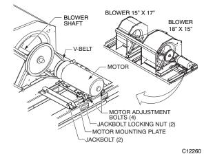
Fig. 4 – Belt Drive Motor Mounting
