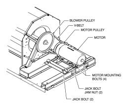
Fig. 9 – Replacing Belt Driven Motor
