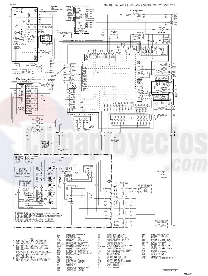
Fig. 77 - 48TC D17 - D28 Control Diagram with Humidi-MiZer®
