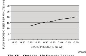
Fig. 68 – Outdoor–Air Damper Leakage
