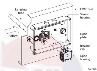
Fig. 42 – Sensor Cleaning Diagram
