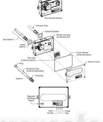
Fig. 36 - Smoke Detector Sensor
