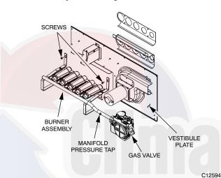
Fig. 53 - Burner Assembly Removal
