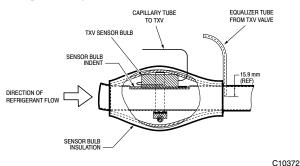
Fig. 21 – TVX Sensor Valve Insulation
