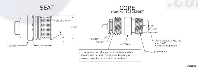
Fig. 15 - CoreMax Access Port Assembly
