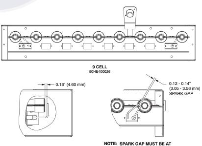
IGNITER AND SENSOR LOCATIONS (BRACKET HEAT COVER NOT SHOWN FOR CLARIY
