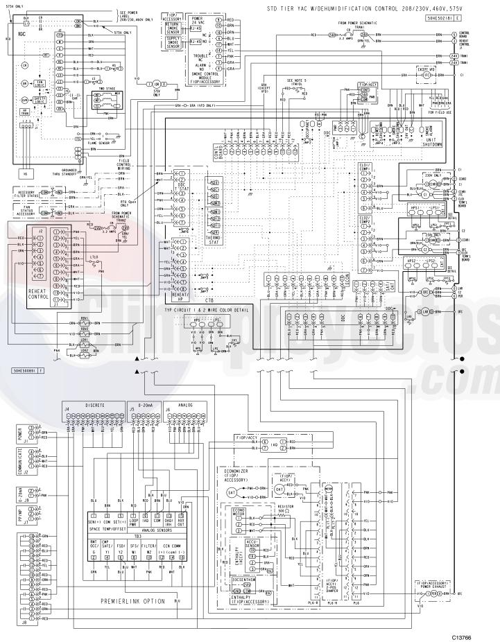
Fig. 82 - PremierLink<sup>™</sup> System Control Wiring Diagram with Humidi-MiZer®
