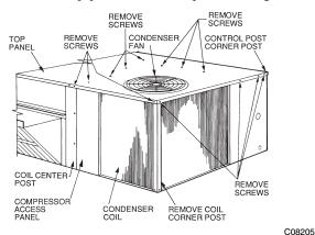
Fig. 12 – Cleaning Condenser Coil
