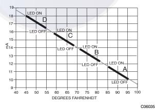
Fig. 67 – Outside Air Temperature Changeover Setpoints
