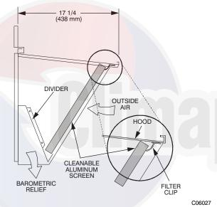
Fig. 3 - Inlet Air Screen Installation
