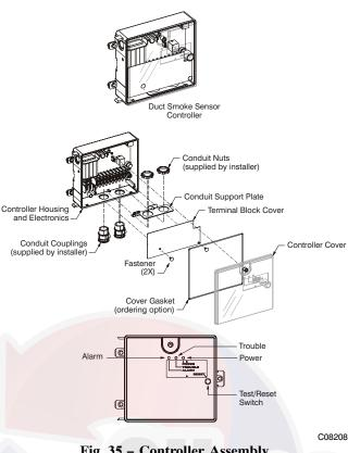
Fig. 35 - Controller Assembly
