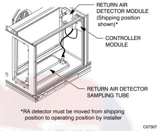
Fig. 38 – Typical Return Air Detector Location
