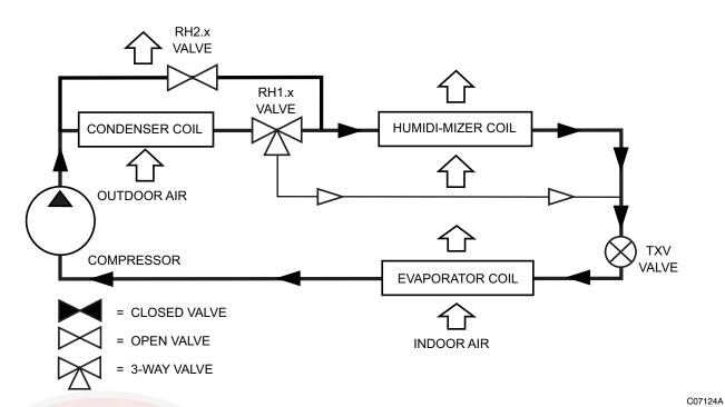
Fig. 19 – Hot Gas Reheat Mode (Reheat 2) – Humidi–MiZer® System
