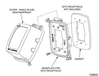
Fig. 34 – Weatherproof Cover Installation
