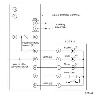
Fig. 41 – Remote Test/Reset Station Connections
