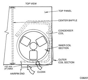
Fig. 14 – Separating Coil Sections
