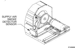
Fig. 37 – Typical Supply Air Smoke Detector Sensor Location
