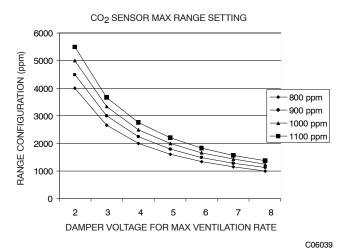
Fig. 72 – CO<sub>2</sub> Sensor Maximum Range Settings
