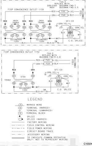
Fig. 33 – Powered Convenience Outlet Wiring
