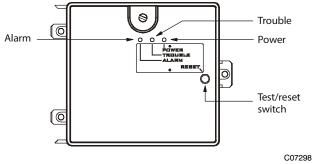
Fig. 43 – Controller Assembly
