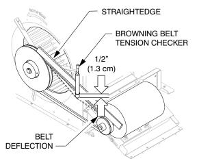
Fig. 5 – Checking Blower Moter Belt Tension
