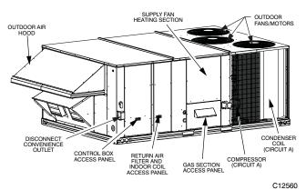
Fig. 1 – Access Panels and Components, Front
