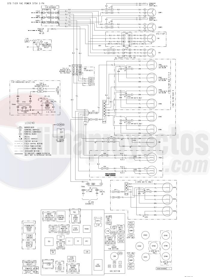
Fig. 76 - 48TC D17 - D28 Power Diagram - 575-3-60
