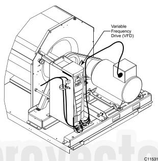
Fig. 8 – VFD Location for 48TC 15–27.5 Units
