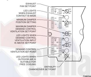
Fig. 66 – EconoMi\$er IV Controller Potentiometer and LED Locations
