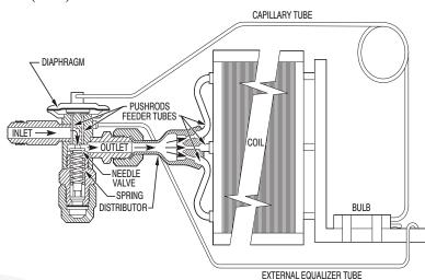
Fig. 20 – Thermostatic Expansion Valve (TXV) Operation
