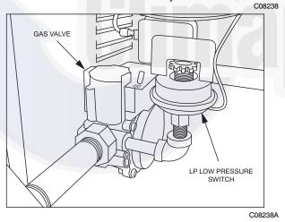
Fig. 49 – LP Low Pressure Switch (Installed)
