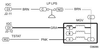
Fig. 50 – LP Supply Line Low Pressure Switch Wiring
