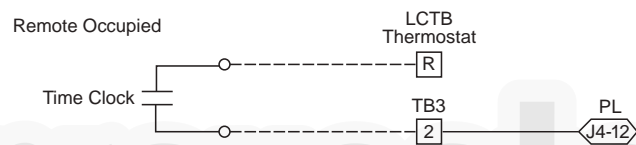
Fig. 61 — PremierLink Wiring Remote Occupied
