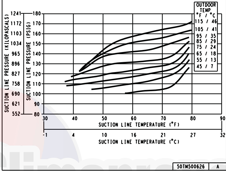
Fig. 27 – Cooling Charging Charts – 50TCQD14, Circuit 2
