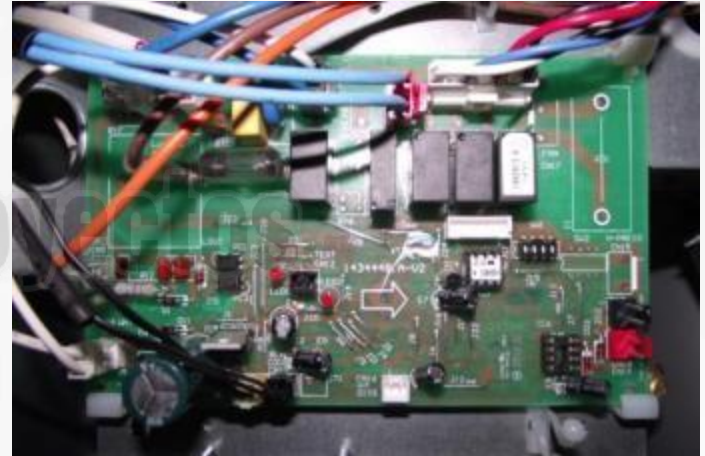
outdoor control board
