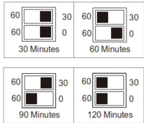
Dipswitch Settings for Selection of Defrost Time
