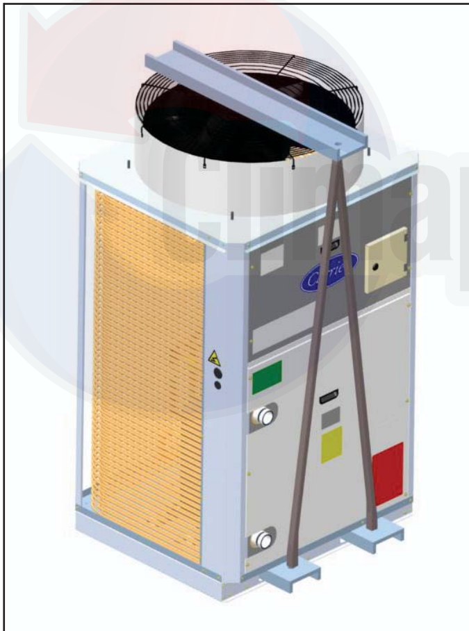
FIG. 2 - Hoisting/Lifting the 30EV / 30EX
