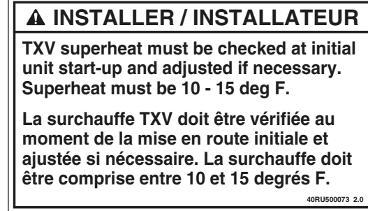
Fig. 20 — TXV Adjustment Label
