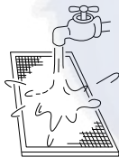
Fig. 8 —Cleaning filter with water or vacuum
